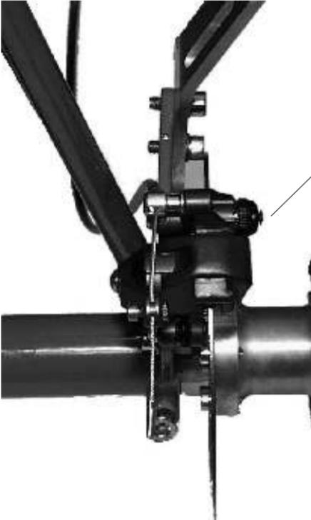
If the brake pads are worn, they must be renewed immediately. Otherwise damage to the brake disc may occur.
