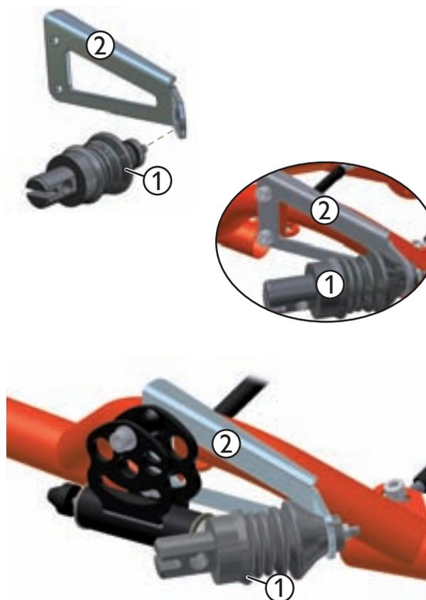
the Kettwiesel. Danger of accident! For curved drawbars, only use the adapter (2) that has been specially designed for this purpose.
